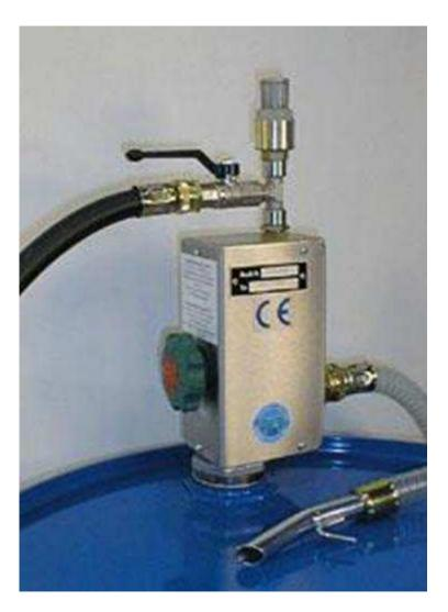
Mixing devices are highly recommended to obtain a homogenous emulsion at the desired concentration.
